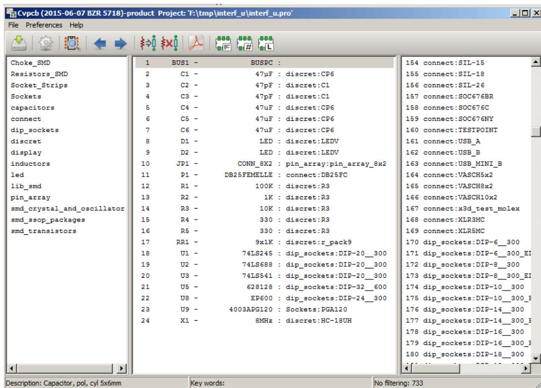
Filtered by list of footprint filters assigned to the selected component. The component filters are listed on the center pane of the status bar at the bottom of the main window.
