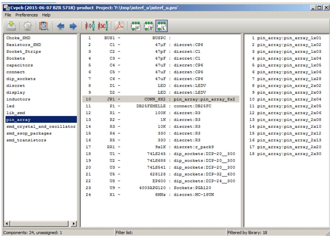
The filtering can be combined to form more complex filtering to help reduce the number of footprints in the footprint pane.
