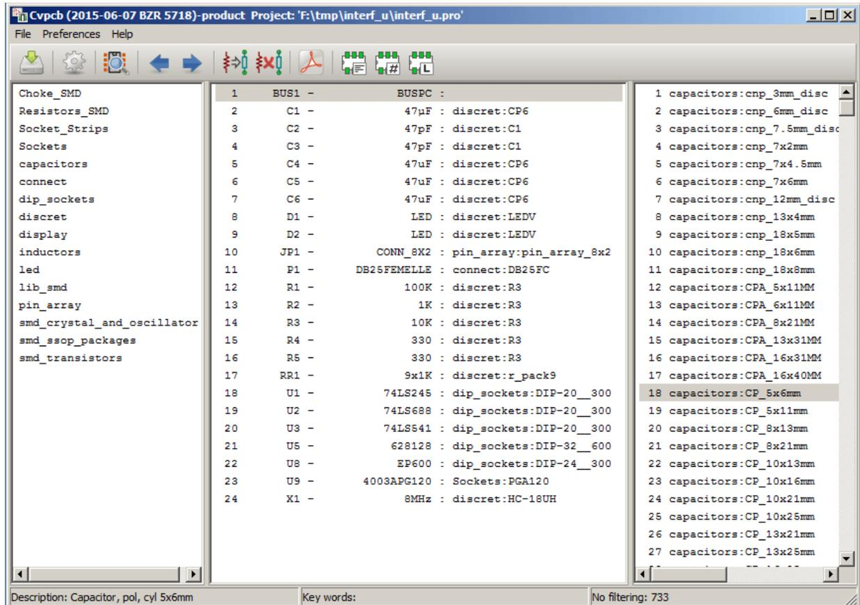
The left pane contains the list of available footprint library file names associated with the project. The center pane contains the list of components loaded from the net list file. The right pane contains the list of available footprints loaded from the project footprint libraries. The component pane will be empty if no netlist file has been loaded and the footprint pane can be also empty if no footprint libraries are found.
